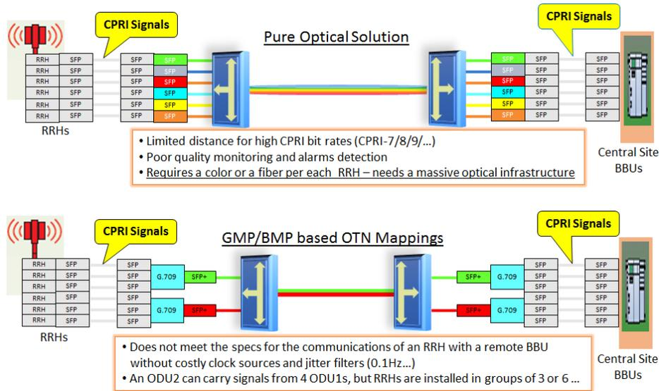
Figure 5: Optical transport technologies for Mobile Fronthaul networks
