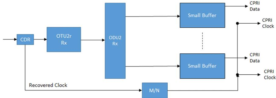
Figure 4: Improved de-mapper; De-mapping of CPRI signals from OTU2r/ODU2r bearers
