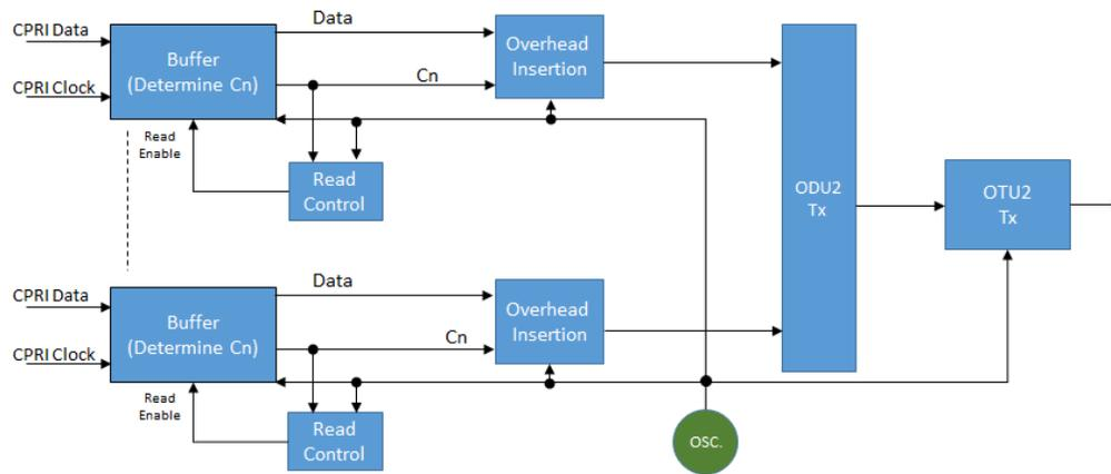
Figure 1: Traditional G.709 mapper; Mapping of CPRI signals to an OTU2 bearer
