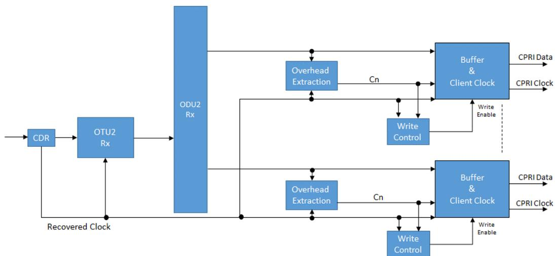
Figure 3: Traditional G.709 de-mapper; De-mapping of CPRI signals from an OTU2 bearer
