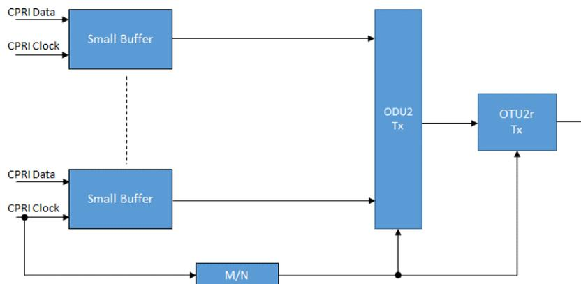
Figure 3: Improved mapper; Mapping of CPRI signals to OTU2r/ODU2r bearers
